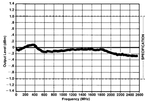
Typical absolute level accuracy. 0 dBm output setting.
